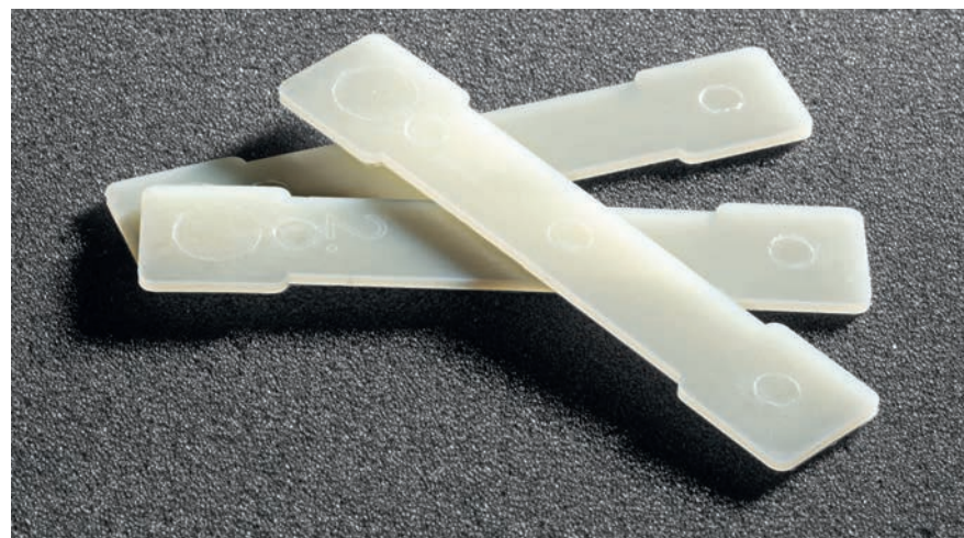
Fig. 7. Shot-weight 4 g, flow-path length 90 mm, wall thickness 2 mm; the "rod" test sample.
