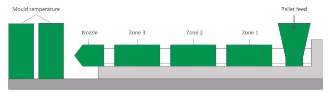
\*For a higher HDT the material can be injected in hot mould but longer cycle times will be required. Please contact BIO-FED for more information.
