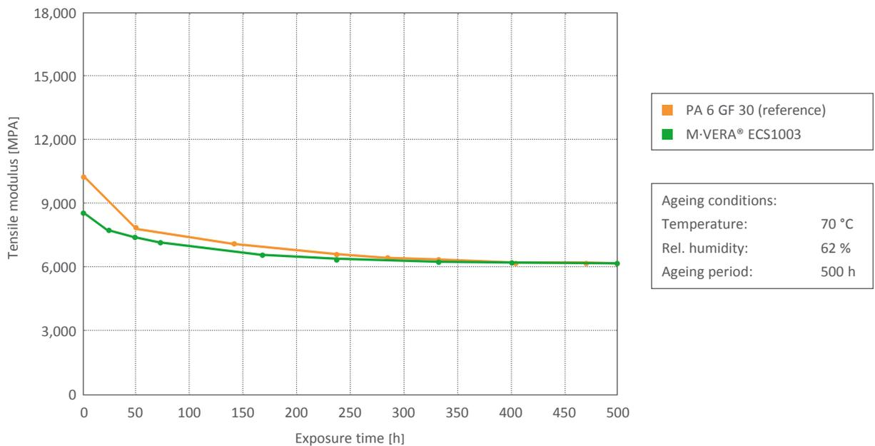
*Following moisture absorption, tensile modulus in M·VERA® ECS1003 decreases significantly less than in PA 6 GF 30*
