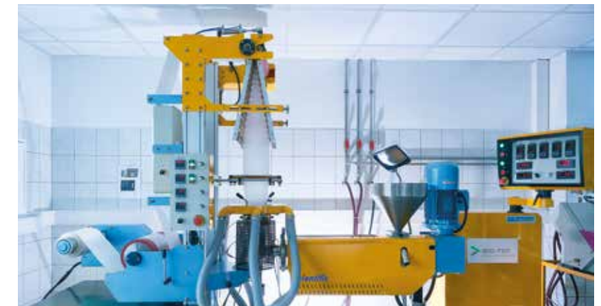
Testing M-VERA® film compounds on our blown film line.
